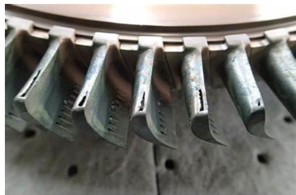
Figure 2. Erosion of turbine blades [29]
