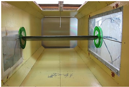
Figure 5. View of the wing section installed and the hot wire sensor inside the test chamber
